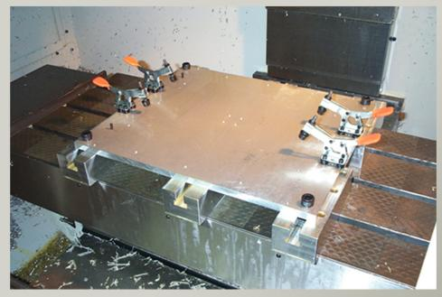
T-Slot Blocks at work. The T-Slot Blocks acts as a support and clamping base for the fixture plate. Fixture plate is wider than the machine table.
