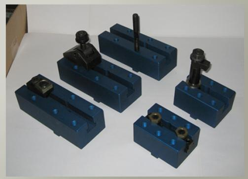
Preload the T-Slot Block with clamps, studs, etc. off the machine table.
